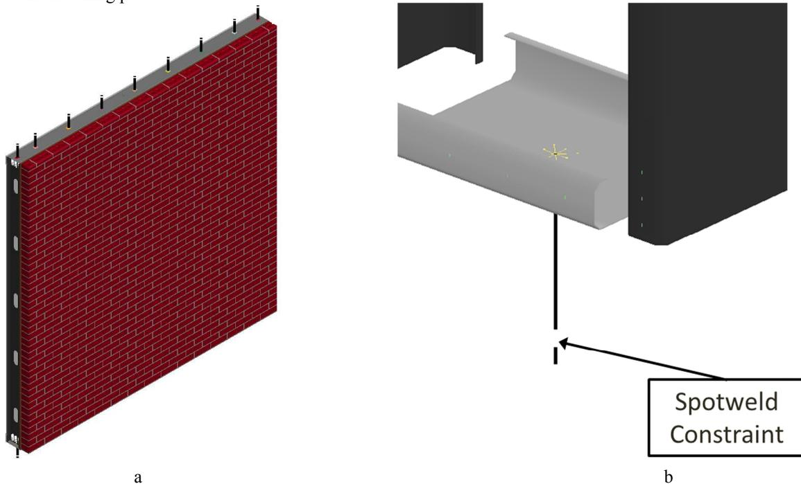
**Figure 2.** Model setup a) overall model view and b) anchor treatment
