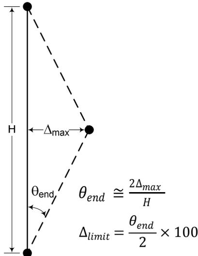
**Figure 6.** Three hinge response mechanism
