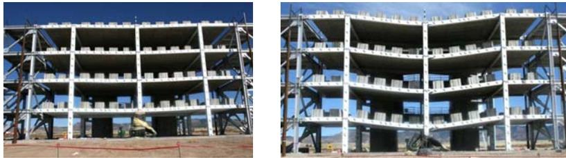
**Figure 7. DTRA/DSTA Full Scale Reinforced Concrete Test Structure**
