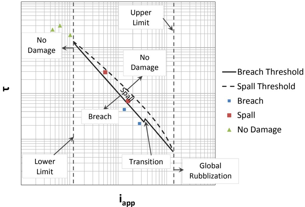
**Figure 8.** Factored Threshold Curves – Circular Cross Section
