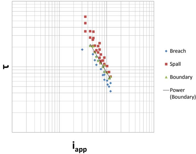
**Figure 7.** Breach Threshold for Contact Detonation on Circular Column Section
