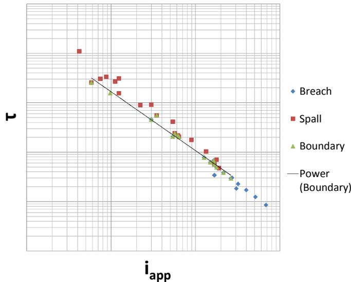
**Figure 6.** Breach Threshold for Close-in Detonation on Circular Column Section
