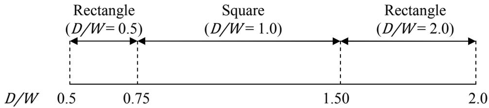
**Figure 9.** Transition Ratios for Square and Rectangular Threshold Curves
