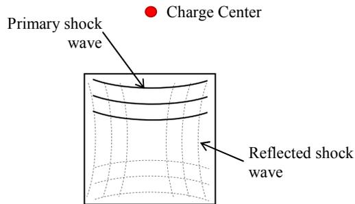
**Figure 3.** Column: 2D Shock Propagation
