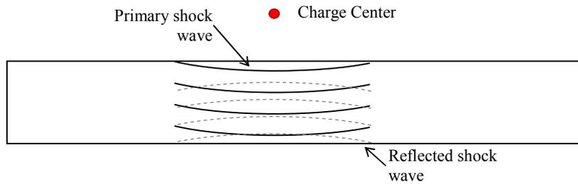
**Figure 2.** Slab or Wall: 1D Shock Propagation
