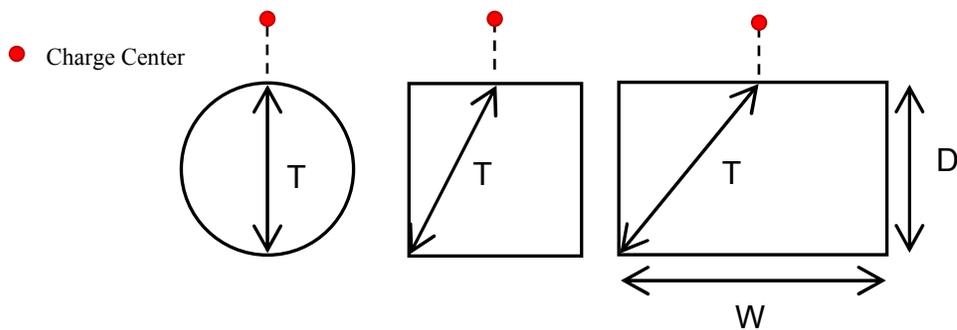
Figure 5. Effective Thickness of Target
