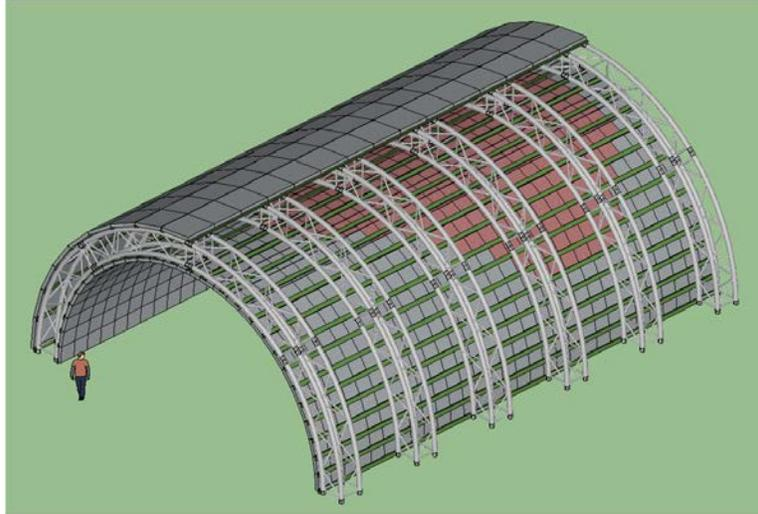
**Figure 7.** Prefabricated Aluminum Truss Arch Structure
