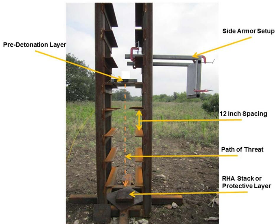
Figure 1. SwRI Welded Test Structure
