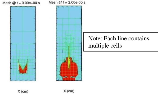
**Figure 6.** Lower Resolution AMR Mesh
