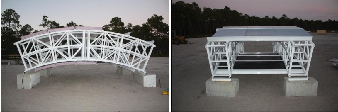
**Figure 9.** Two Arch Sections with Pre-detonation and Armor Layers Covering Half of the Test Sample.
