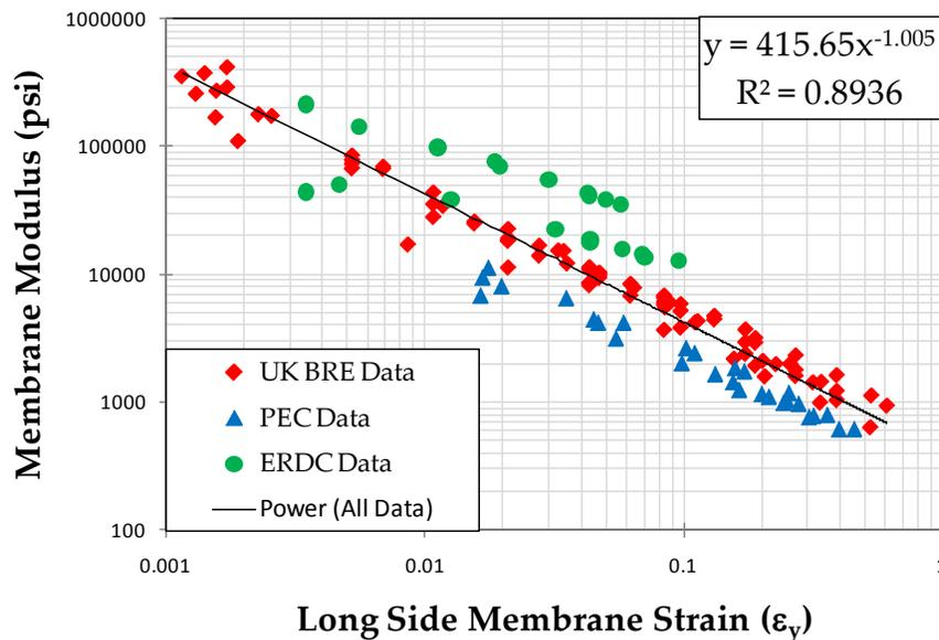
Figure 1-2. Results of Regression Analysis for Development of Refined Membrane Modulus Expression
