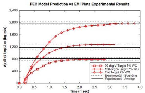
Figure 10. ALE Imparted Momentum for EMI Tests with 7% Water Content, PEC Soil Model
