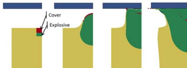
Figure 15. Reduced Density and Water Content above Explosive, EMI Flat Plate
