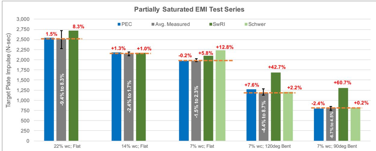
**REVISED** Figure 9. Comparison of EMI Experimental Impulses with Models by PEC, SwRI, and Schwer [15]
