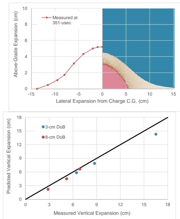
Figure 6. 8-cm DOB Soil Expansion Simulation for Hybrid SPH-ALE Modeling Strategy; Measurements Adapted from (17)
