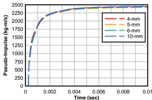
Figure 14. Impulse Histories for Different ALE Element Sizes, EMI Flat Plate 7% Water Content
