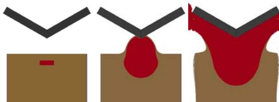
Figure 7. ALE Response Evolution for EMI 120-deg Bent Plate Impact Simulation
