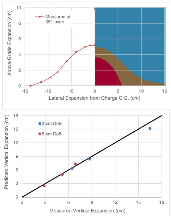
Figure 4. 8-cm DOB Soil Expansion Simulation for ALE Modeling Strategy, PEC Soil Model; Measurements Adapted from (17)
