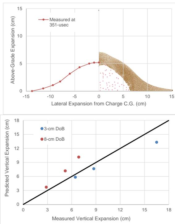
Figure 5. 8-cm DOB Soil Expansion Simulation for SPH Modeling Strategy; Measurements Adapted from (17)
