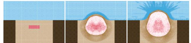
Figure 12. Unstable SPH Air to Soil Particle Contact Caused by Shooting Rogue Particles
