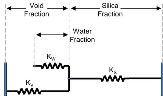
Figure 1. Element Schematic of Three-Spring Compaction Model
