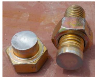
(b) Bolt shear fracture
