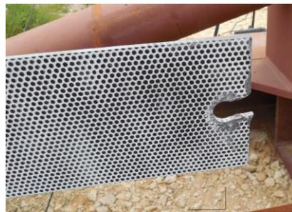
(a) plate tear-out failure
